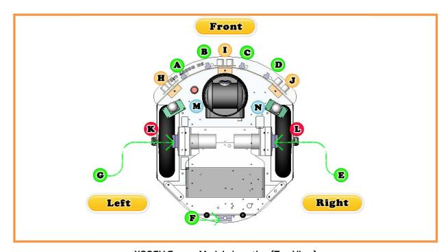
X805V Sensor Module Location (Top View)
