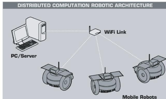
With its integrated high bandwidth (11Mbps) WiFi 802.11 wireless module, the system can upload all sensor data (including encoder sensor readings) to a PC or server at rates in excess of 10Hz. Similarly, streaming audio (8Hz x 8bits) and video (up to 4 fps) either for direct monitoring or for
